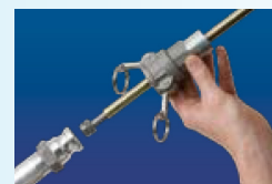
Complete Service Work, Restore System Supply, Remove Bagging Assembly, Install Plug & Disassemble System
