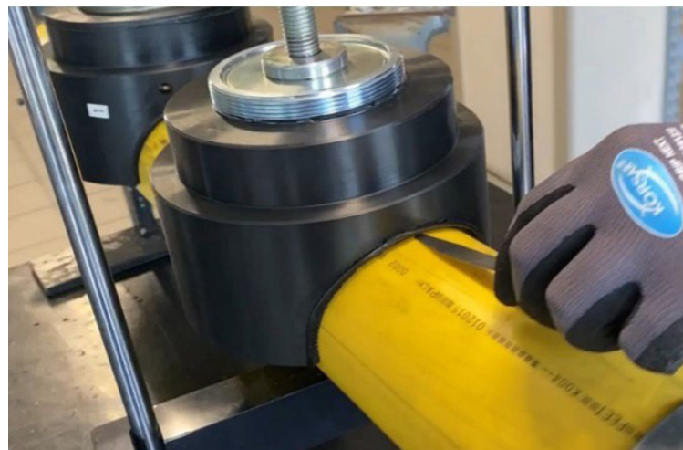
Figure 1. Guage Checks for Shur Stop 4"-12" Fittings (0.3mm Metal Feeler Guage
